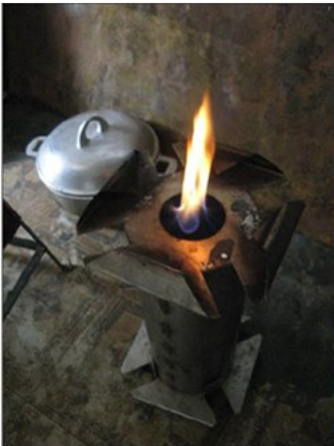
Left: The blue flame indicates that the Haiti Lucia stove is burning cleanly and efficiently.
