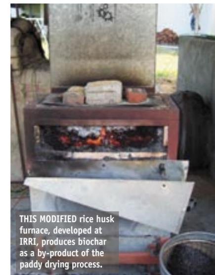
THIS MODIFIED rice husk furnace, developed at IRRI, produces biochar as a by-product of the paddy drying process.
