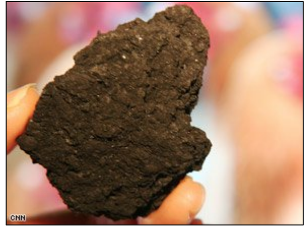
Fig. 2 Biochar's high carbon content and porous nature can help soil retain water, nutrients, protect soil microbes.
